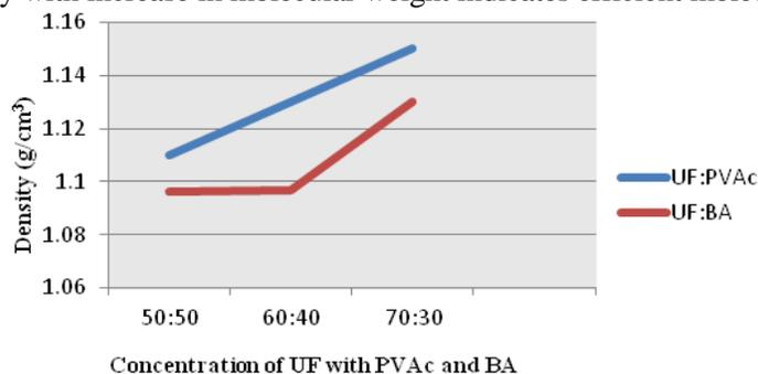
**Figure 2. Effect of PVAc and BA Concentration on the Density of UF**
