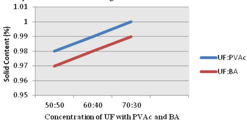
Figure 7. Effect of PVAc and BA Concentration on the solid content of UF
