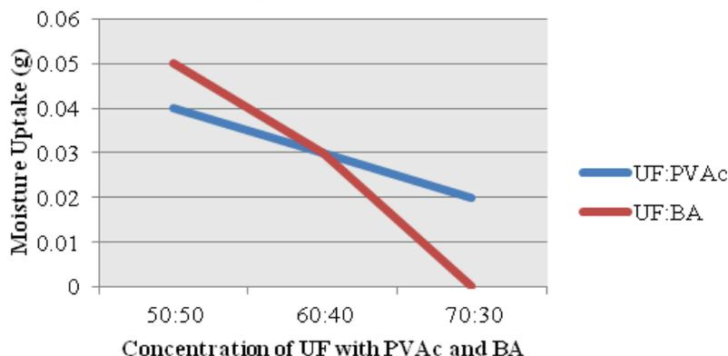
Figure 6. Effect of PVAc and BA Concentration on the moisture uptake of UF
