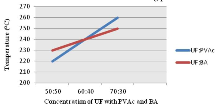
**Figure 3. Effect of PVAc and BA Concentration on the Melting point of UF**
