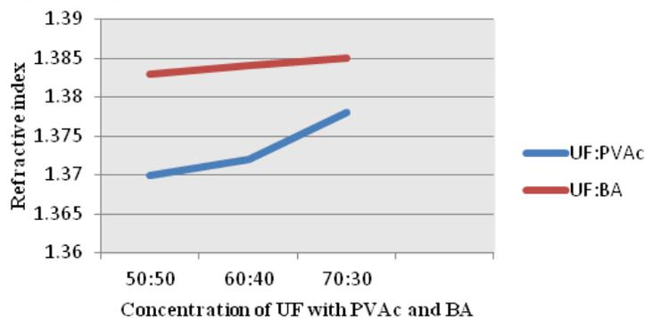
Figure 5. Effect of PVAc and BA Concentration on the refractive index of UF
