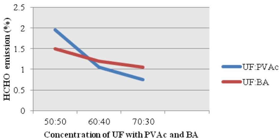
Figure 8. Effect of PVAc and BA Concentration on the HCHO emission of UF
