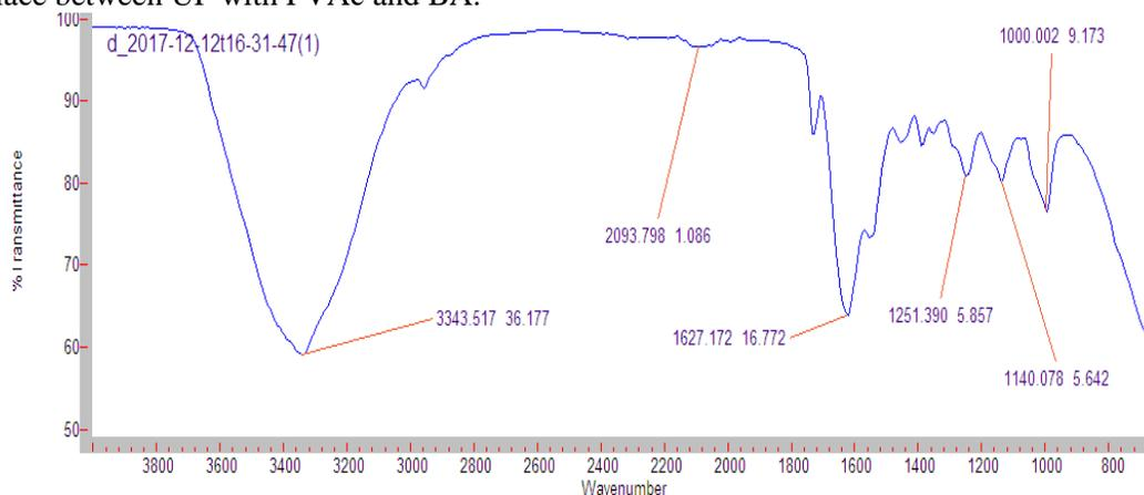
**Figure 11. IR Spectra of UF: BA**
