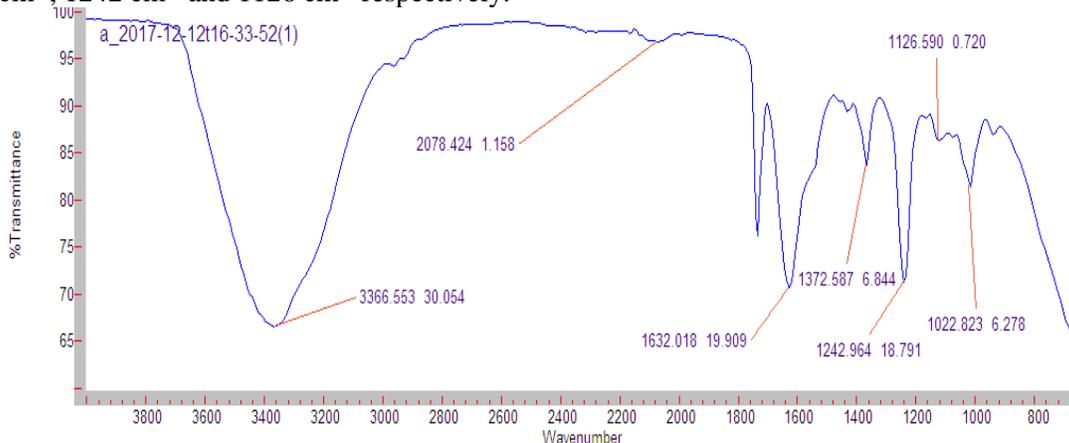
**Figure 10. FT-IR Spectra of UF:PVAc**
