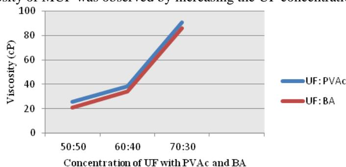
**Figure 1. Effect of PVAc and BA Concentration on the Viscosity of UF**
