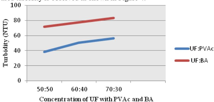
**Figure 4. Effect of PVAc and BA Concentration on the Turbidity of UF**
