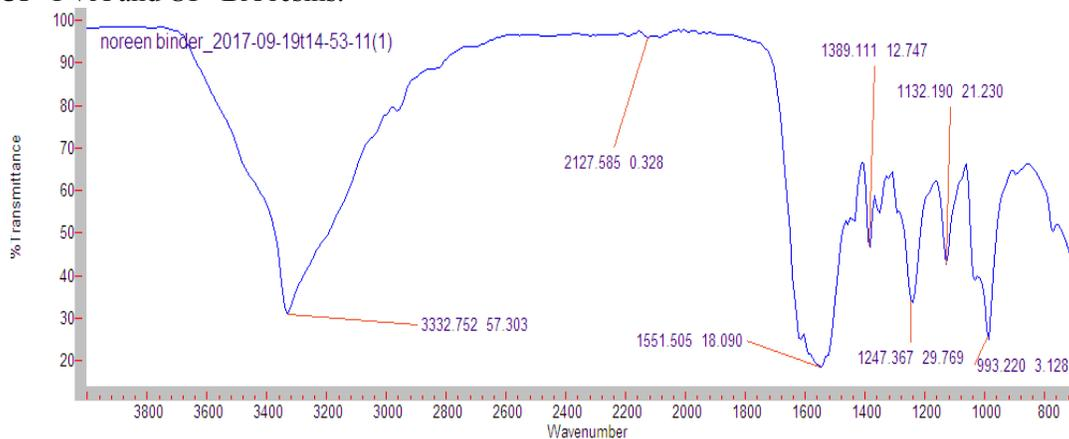
**Figure 9. IR Spectra of UF**
