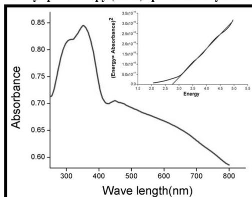
Figure 5. UV-Vis absorbance of synthesized Ag/ZnO nanoparticles. Inset picture indicates the band gap energy of the nanoparticles.
