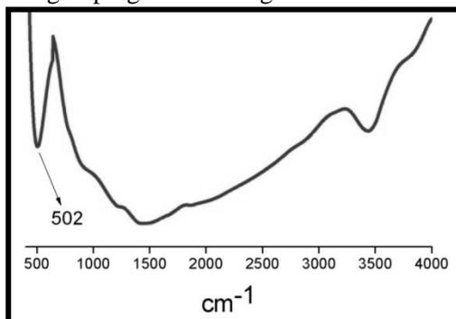
Figure 1. FT-IR spectrum of synthesized Ag/ZnO nanoparticles.
