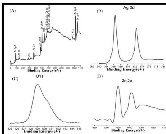
Figure 3. (A) XPS full spectrum of synthesized Ag/ZnO nanoparticles; (B) Ag 3d spectrum; (C) O 1s spectrum and (D) Zn 2p spectrum.
