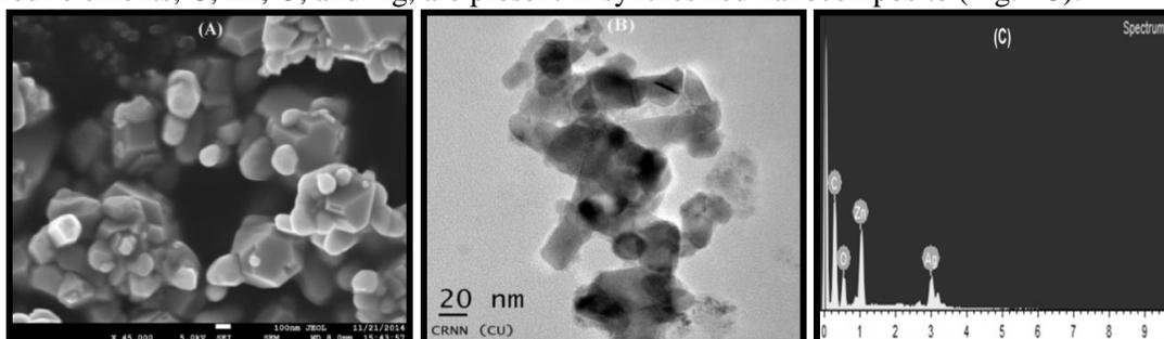
Fig.-4 (A) Scanning electron microscopy (SEM) image (B) Transmission electron microscopy (TEM) image and (C) Energy-dispersive X-ray spectroscopy (EDX) spectrum of synthesized Ag/ZnO nanoparticles.
