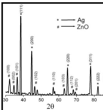
Figure 2. XRPD spectrum of synthesized Ag/ZnO nanoparticles.
