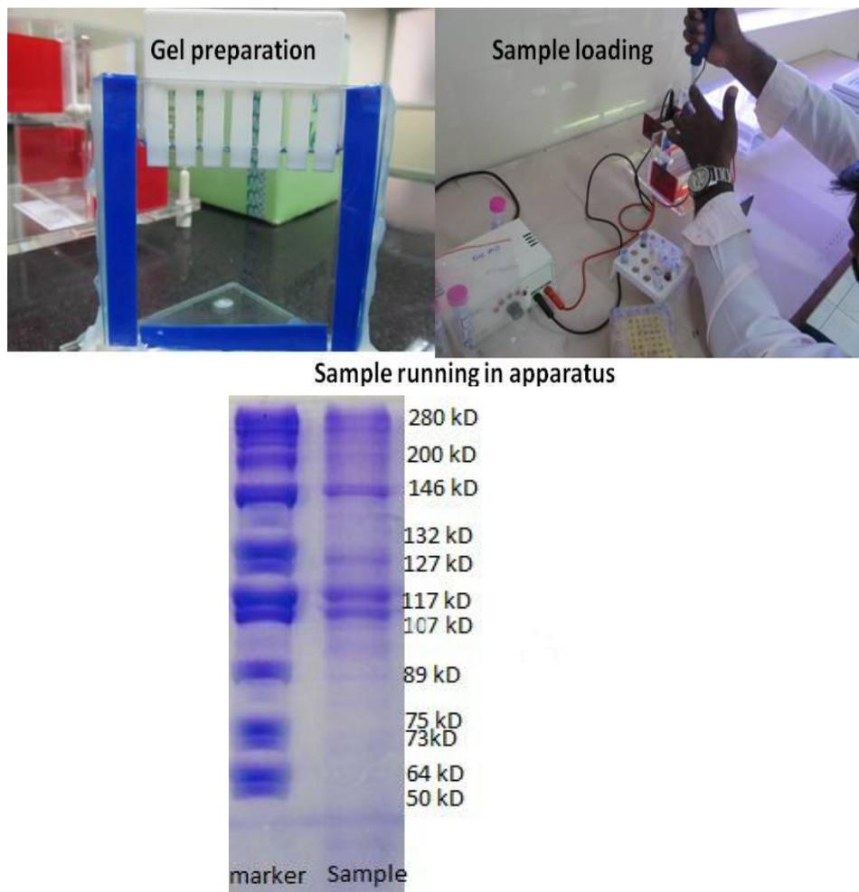
Fig- 5 SDS-PAGE Electrophoresis image
