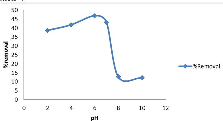
Figure: 1.3 Change in percentage adsorption of Nickel (II) with time at different pH
