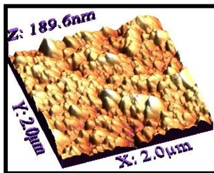
Fig. 3 AFM micrograph of Al: CdO (2%) thin film.
