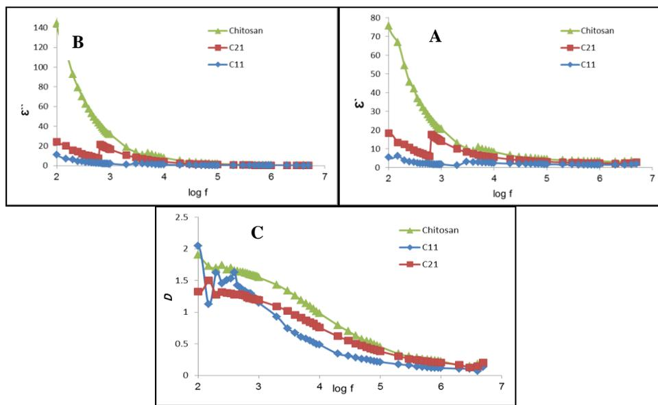
**Fig.3: (3a) Dielectric constant as a function of frequency and (3b) Dielectric loss  $\epsilon''$  (3C) Dielectric loss tangent as a function of frequency for pure chitosan, C11 and C21 films at room temperatures**
