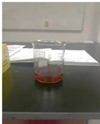
**Figure 5: Crude glycerol obtained from palm oil biodiesel production.**
